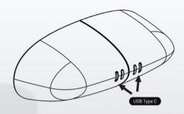
To Power up the Speaker, simply plug in Type C Cable into Speaker back side and plug USB A into the power supply or wall charger.
